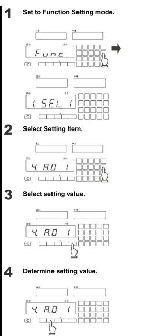
Keep pressing [MODE] key for 3 to 4 seconds, then release key when " $\Gamma_{\mu} \cap \Gamma$ " is displayed.
