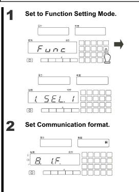
Keep pressing [MODE] key, and release key when " $F \Box \cap c$ " is displayed.
