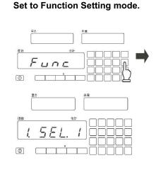
Keep pressing [MODE] key for 3 to 4 seconds, then release key when  ${}^{"}F_{\mu} \cap C$ " is displayed.
