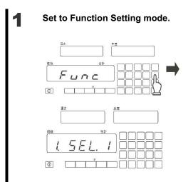
Keep pressing [MODE] key for 3 to 4 seconds, then release key when " $\overline{}^{\mu} \, \square \, \square \, \square^{n}$ " is displayed.
