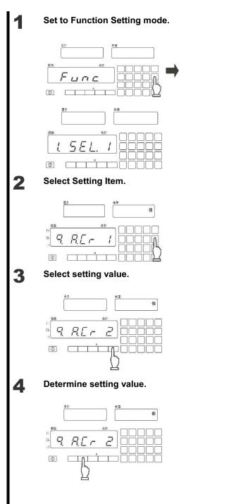
Keep pressing [MODE] key for 3 to 4 seconds, then release key when " $F \sqcup n \subset$ " is displayed.
