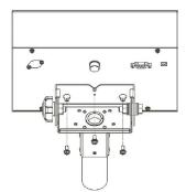
Using 2.5mm Hexagon Head wrench, fix Pole to pole base using Pole Fizing screws.
